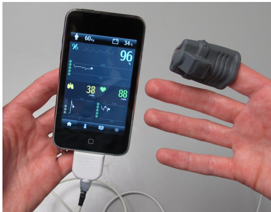
Figure 1: First prototype of the Phone Oximeter
