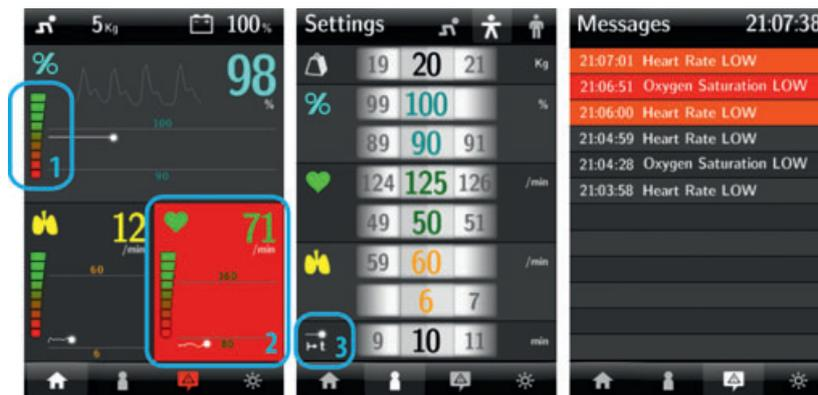
**Figure 3** The second Phone Oximeter graphical user interface prototype as used in Phase II of the study. Visual changes made to the interface are highlighted in blue: (1) new signal quality indicator; (2) improved visual alert for alarms; and (3) improved icon for the trend line indicator.
