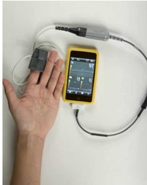
**Figure 1** The Phone Oximeter prototype consists of an Apple iPod Touch hardwired to a Nonin Xpod OEM pulse oximeter module. The *Home* tab displays PPG (photoplethysmograph) and  $S_pO_2$  (oxygen saturation) (top), respiratory rate (bottom left) and heart rate (bottom right).
