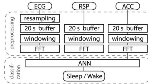
Fig. 1. Overview of the sleep/wake classification algorithm. Raw ECG, RSP and ACC signals are recorded and stored in a buffer for 20 s. Then a window function is applied and a short-time fast Fourier transformation (FFT) is used to calculate the spectral power density. The resulting frequency data are fed to a feed-forward ANN with a tangent-sigmoid transfer function. A symmetric classification threshold separates the ANN output into sleep or wake.
