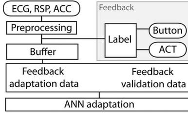
Fig. 2. Overview of the data flow for the automatic labeling of sleep/wake for the cardio-respiratory and accelerometer data (ECG, RSP, ACC) that were used for the adaptation of the ANN classifier. *A priori* label information is obtained from button and activity (ACT) data.
