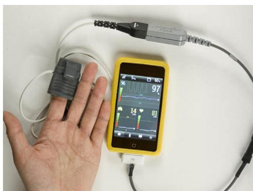
Figure 1. The Phone Oximeter™ interfacing a microcontroller-based pulse oximeter module with a smartphone.
