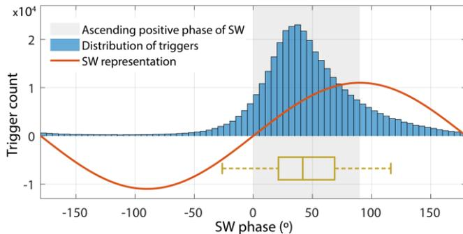
Fig. 5. The triggers are distributed around the ascending positive phase (shaded) of SW ( $n = 93$  recordings). The boxplot (without outliers) illustrates the statistical phase distribution of the triggers. During negative phase the number of triggers is minimized.
