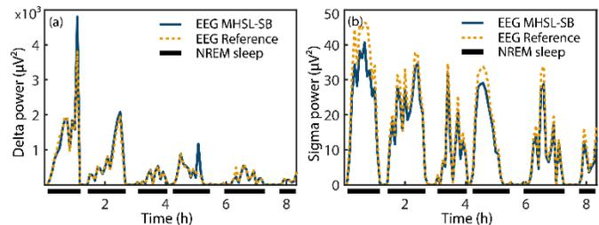
Fig. 3. Mean square signal power in the (a) delta and (b) sigma frequency bands during detected NREM sleep episodes (black blocks) showed high correlation between the MHSL-SB and reference device.
