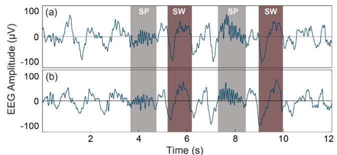
Fig. 4. Typical NREM sleep patterns such as spindles (SP) and slow waves (SW) are clearly apparent in the EEG during NREM sleep in the (a) reference and (b) MHSL-SB device.
