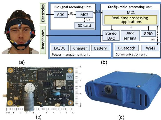
Fig. 1. The MHSL-SB (a) headband, (b) system architecture, (c) printed circuit board, and (d) portable casing. When the headband cable was plugged into the analog connector, the system autonomously started biosignal recording and processing without additional user input.
