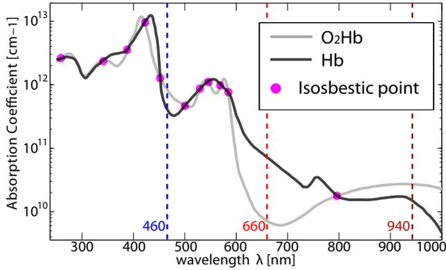
Fig. 1. Absorption curves for O<sub>2</sub>Hb and Hb over the full visible and near IR spectrum. Circles mark isosbestic points where absorption properties for both mediums are equal. Created with data from [15].
