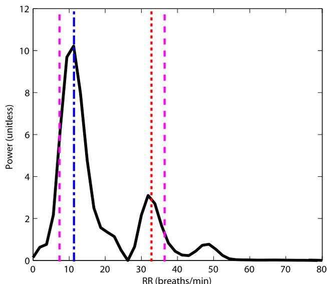
Fig. 6. Example of high power in a low RR band where reference RR is high (dotted line). The dashed lines represent the RR selection range, the dot-dash line is the selected RR by the algorithm.
