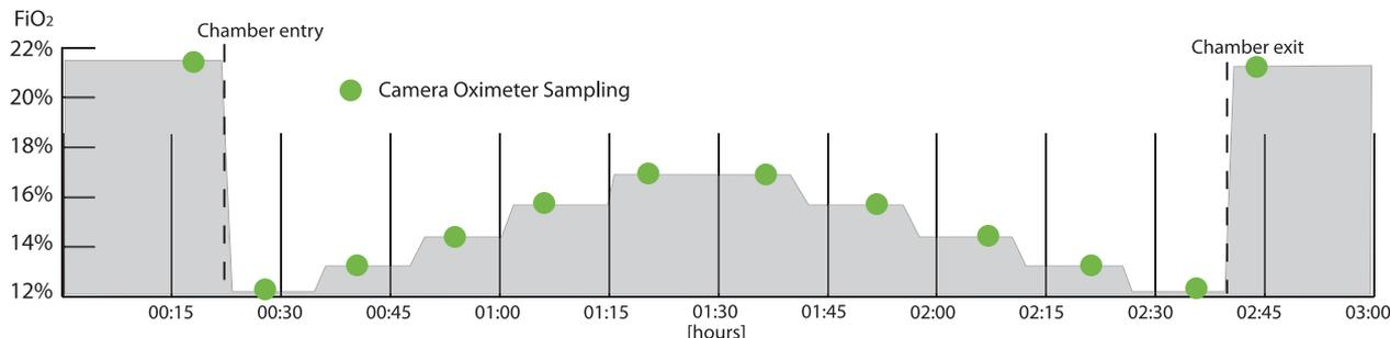
Fig. 1. Experimental setup with changing  $\text{FiO}_2$  input. The green dots represent time points when sampling with the Camera Oximeter was performed and reference RR was measured using a capnometer. Reference pulse oximetry was recorded throughout the entire experiment.
