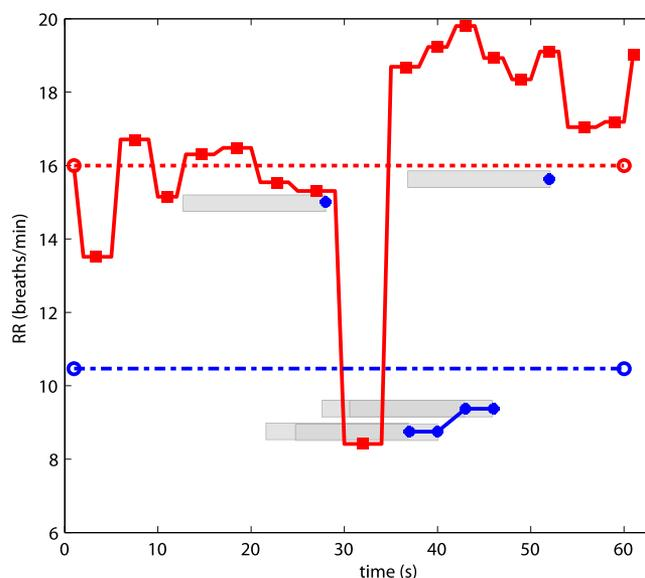
Fig. 7. Example of high variation in RR within 60 s. The estimated RR (dot-dash blue) is lower than the reference RR (dotted red) as valid estimation was primarily found for a window where RR was low. The window size was 16 s (grey boxes). Instantaneous RRs are shown as filled squares (reference) and circles (Camera Oximeter).
