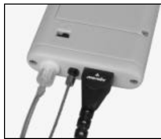
Nasal cannula, optical fiber, and oximeter connections.
